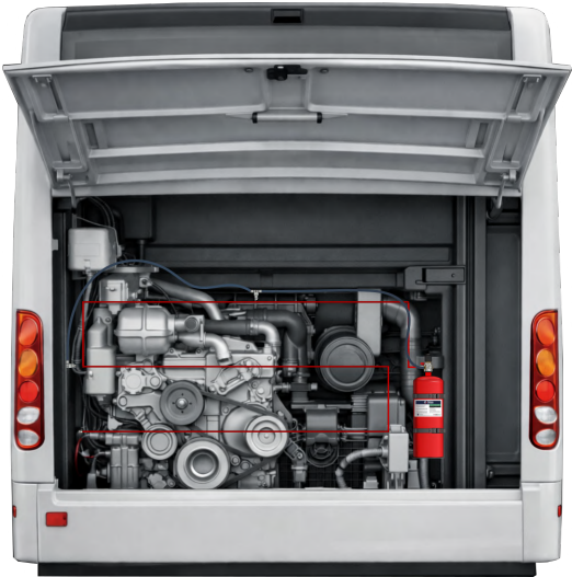
ILP System in Engine Bay w/ Multiple Nozzle Config.
